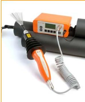
The high voltage test method detects flaws in a non-conductive coating applied on to conductive substrates. The voltage is set so that, if the coating is electrically weak in an area, there is sufficient voltage to breakdown the gap between the high voltage probe and the conductive substrate.
