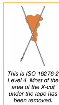
*This is ISO 16276-2 Level 4. Most of the area of the X-cut under the tape has been removed.*
