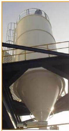
Silo made from vitreous enamelled steel sheets.
