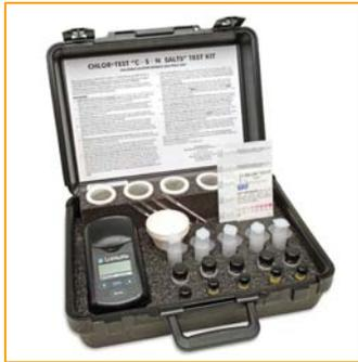
The Elcometer 134 CSN Test Kit is ideal for trouble free testing of chlorides, sulphates and nitrates.
