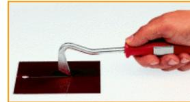
adhesion to it. This can be investigated using a scratching tool such as the Elcometer 1537.
